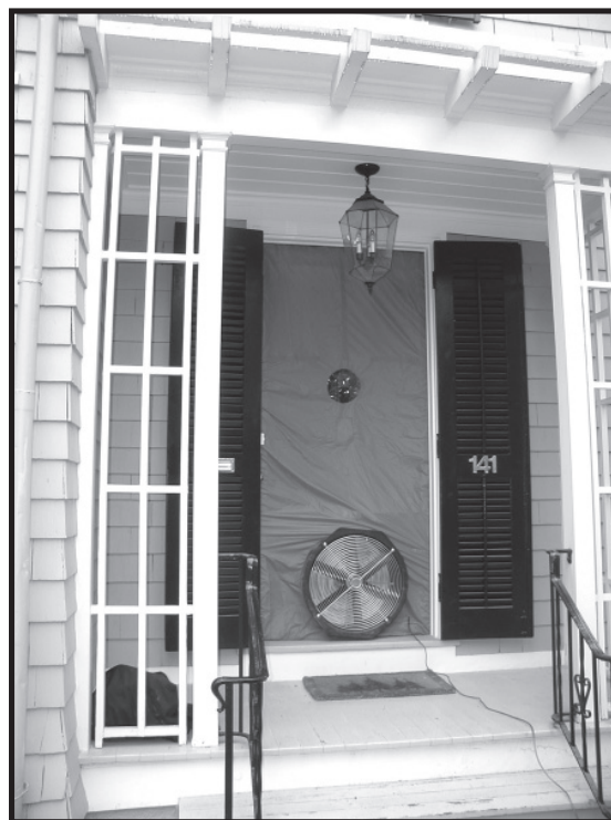
A Blower Door Test can determine a house's air loss and overall efficiency. Photo courtesy of the author.
